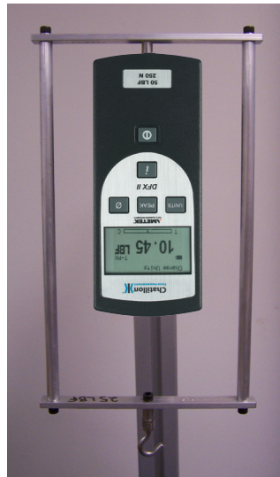
Shown: a correct compression calibration setup using a hanger fixture.
