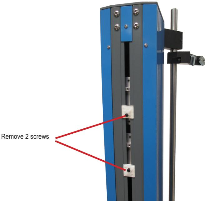
The two (2) arm assemblies can now be fitted with the screws provided (as shown below). Ensure the arm assemblies are properly located and secured.
