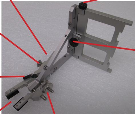
The sample can be loaded on the LS test machine between the appropriate grips as shown below. Once the sample is in the desired position and the arms aligned horizontally with the sample rotate the extensometer towards the sample until the knife edges are aligned vertically with the sample and the arms aligned to each other by the gauge length block being firmly sandwiched between the arms.
