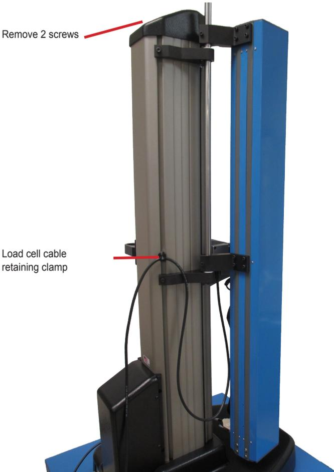
Remove the transit screws from the column. Two (2) screws are found at the back 95mm and 160mm up from the base holding the counter weights.
