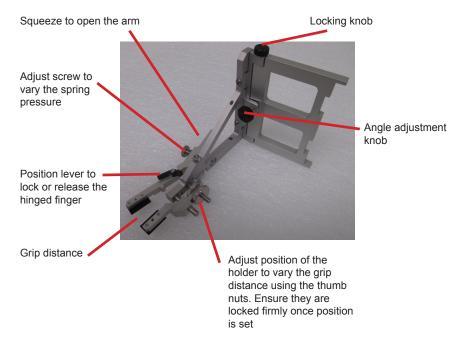
The sample can be loaded on the LS test machine between the appropriate grips as shown below. Once the sample is in the desired position and the arms aligned horizontally with the sample rotate the extensometer towards the sample until the knife edges are aligned vertically with the sample and the arms aligned to each other by the gauge length block being firmly sandwiched between the arms.
