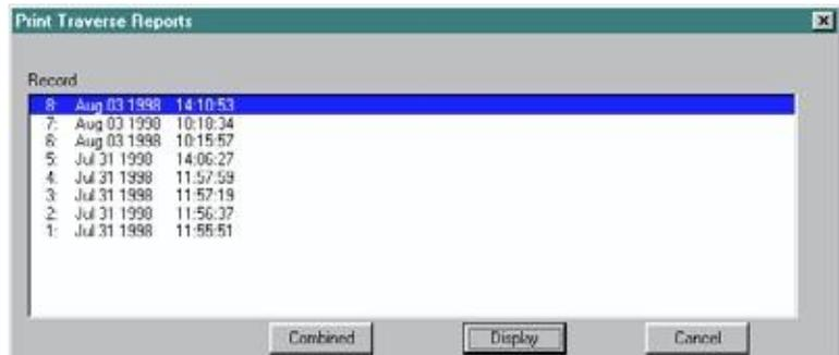
There are three types of Multiple Reports: Graph, Chart, and Display. Graph shows every traverse in the file simultaneously. The Chart Report shows a Graph of the Case depths plotting the case depths side-by-side. The Display Report shows the case depths in a tabular format
