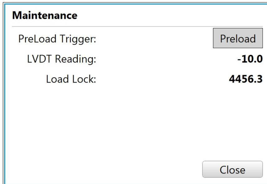
For a motorized machine, the **Maintenance** screen provides an on/off indicators that activate (change from grey to green) at the **PreLoad Trigger**, **Home** position and **Full Load** position, and numeric readouts for the **Depth LVDT Reading** and the **Load Lock** position.
