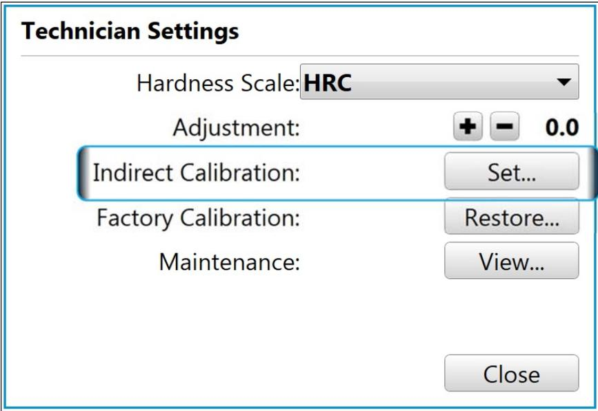
The **Factory Calibration Restore** function allows the technician to remove any previously performed Indirect Calibrations and recovers the system to the original Factory Calibration settings, it's prompted by a confirmation screen to accept or cancel this selection.
