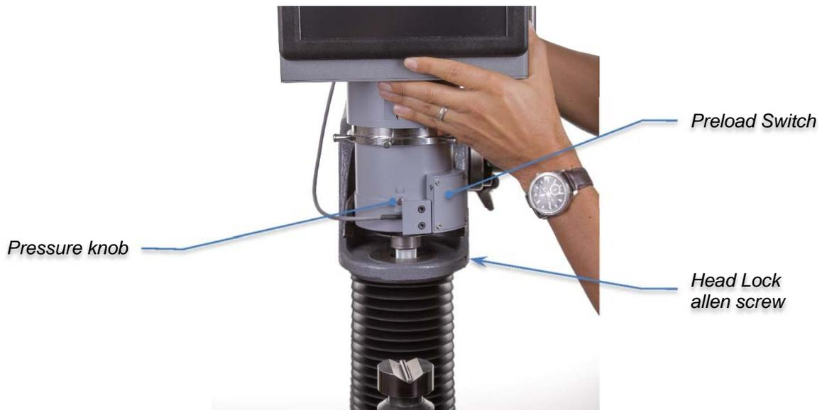
*Installing the Test Head*
