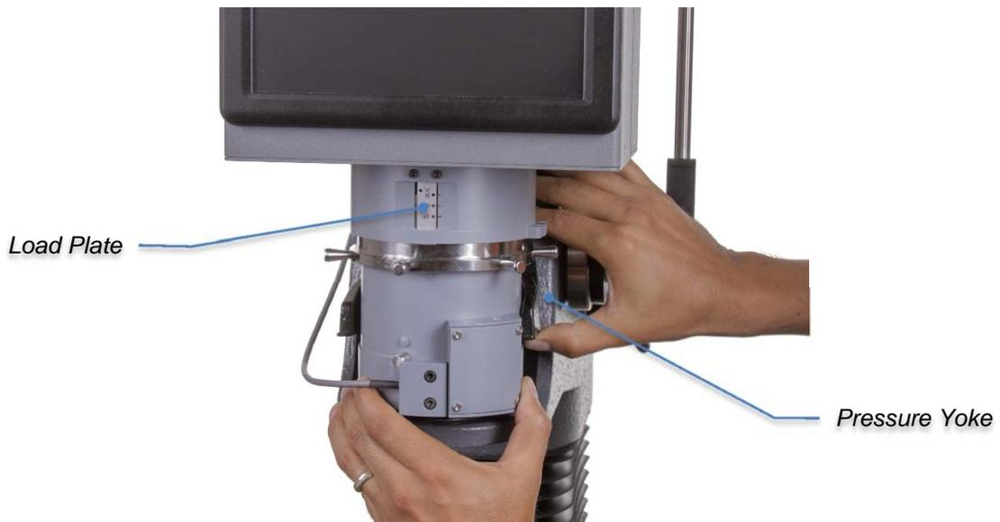
*Installing the Test Head*
