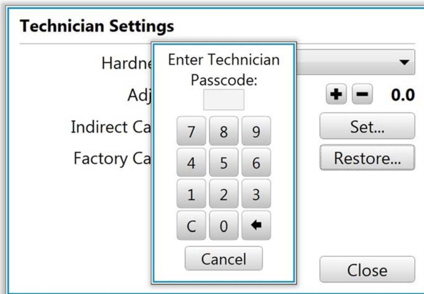
After a successful entry the technician can select the Indirect Calibration **Set** tab to access this function, the **Indirect Calibration** screen allow the selection of a **Hardness Scale** to calibrate.
