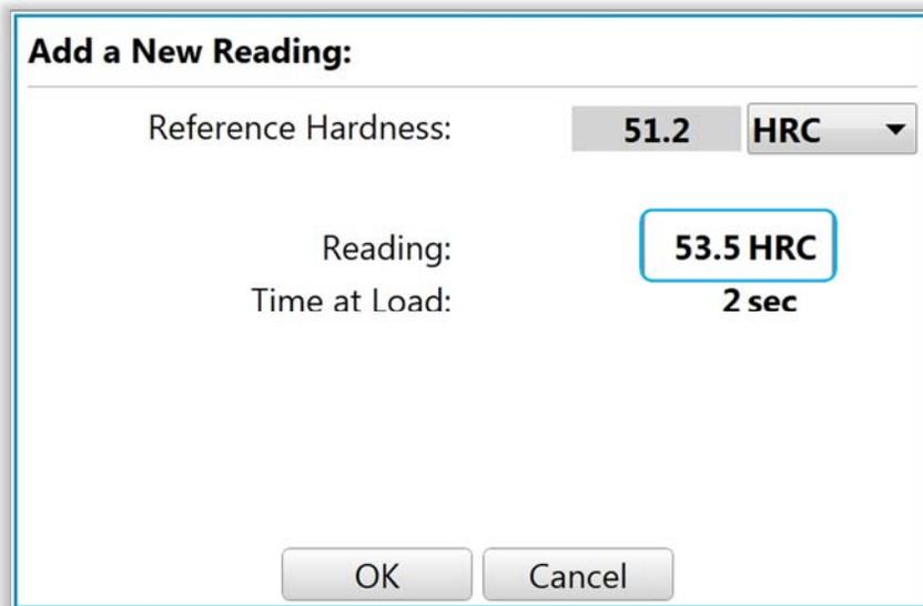
When the first measurement is completed, the **Indirect Calibration** screen will appear with the data grid listing the Reference value, the actual Reading and the Scale used.
