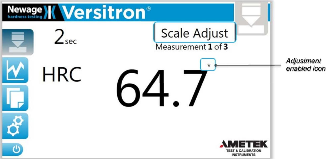
The **Indirect Calibration** option allows a qualified technician to indirectly calibrate the equipment by establishing a new profile set of data points per a specific hardness scale, indenter type or machine (both) using a multi set of scale hardness reference blocks. This process should only be performed by a knowledgeable technician, as it can drastically affect measurement accuracy. This process is not required for normal operation.
