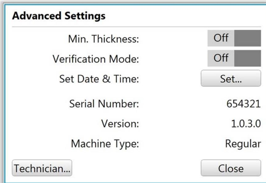
The **Minimum Thickness** function is On/Off selectable. When enabled, it uses the minimum thickness value for a corresponding hardness in the respective scale. See Minimum Thickness reference chart in section 10.2.
