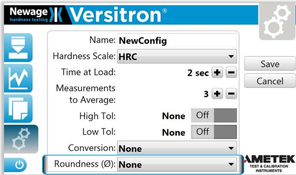
A roundness icon and roundness correction will display on the **Test Screen** reading when this function is enabled.
