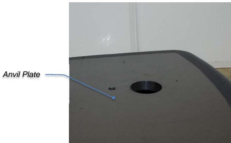
6. On large work pieces, use the clamping shield to secure parts. Otherwise, maintain a distance between indenter and work piece at approximately 1/16". Maximum vertical capacity without anvil stage is 16-1/2" (420 mm) (standard unit). Maximum horizontal reach is 8-1/2" (215 mm). Other T-stand vertical capacities are available up to 36". Use the clamping shield on larger openings to reduce excessive deflection.
