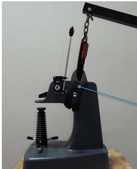
*Ensure the sling is wrapped around this area of the machine (as shown).*
