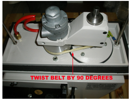
Shown: Polymer grinder top cover and belt
