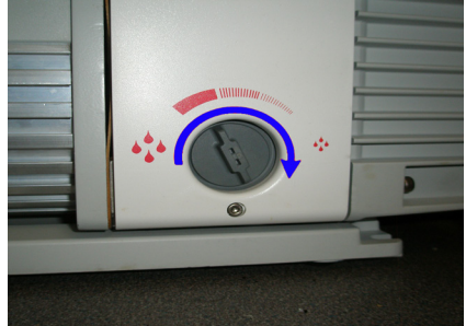
Shown: Rotate mode selector fully clockwise for High Vacuum mode
