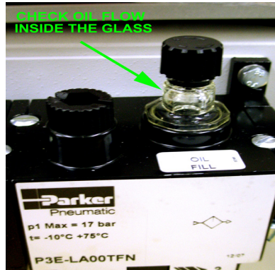
Shown: Check oil drop rate
