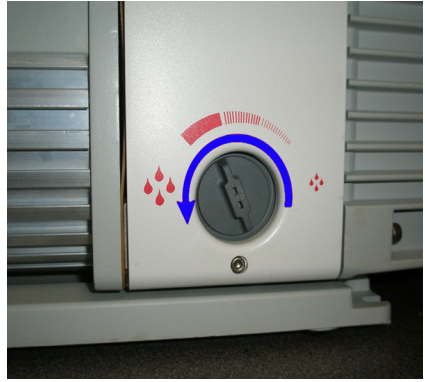
Shown: Turn the mode selector fully counter clockwise
