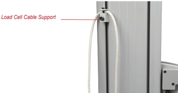
The Load Cell Cable Support can be adjusted up or down on the TA1 Column Extrusion using a 5mm Hex Key. Ensure there is plenty of length in the cable so that the crosshead can travel without pulling the cable assembly.
