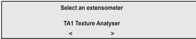
The left and right arrow ( < > ) Soft Keys will scroll through the list of currently connected extensometers, (theoretically a maximum of 4 with the internal crosshead position always being listed as one of these). The internal crosshead position extensometer is displayed as the TA1 texture analyser, i.e., TA1. Press the **ENTER** key to select the displayed extensometer.
