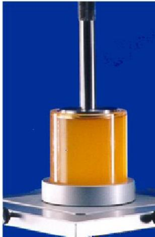
*Back Extrusion Food Cell (Part No. FG/BEC)*
