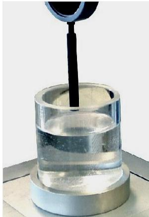
*Cylinder Probe Threaded to Load Cell*
