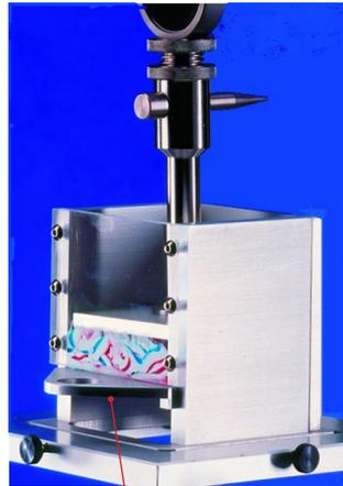
*Extrusion Testing Cell Fixture*
