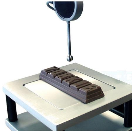
*Ball Probe Threaded to Load Cell*
