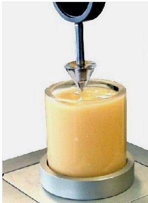
*Cone Probe Threaded to Load Cell*
