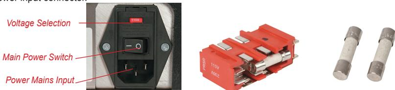
The TA1 machine uses two ceramic high breaking capacity type fuses (20mm x 5mm) as shown above. The two fuses are assembled into the power entry module fuse block as shown above.
