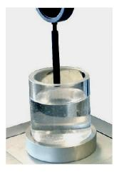
Cylinder Probe Threaded to Load Cell
