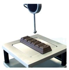
Ball Probe Threaded to Load Cell
