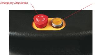
Safeline Button When illuminated, the safeline switch is open. There is no crosshead movement or motor control. Depress the button to close the switch and allow for motor and crosshead movement.
