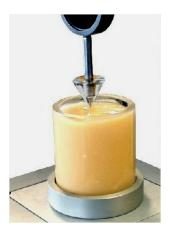
Cone Probe Threaded to Load Cell
