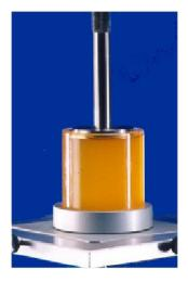
Back Extrusion Food Cell (Part No. FG/BEC)
